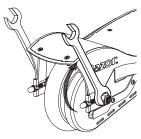
**3** Once the tension is correct, tighten the axle bolts. Test ride the scooter. Readjust as needed.
