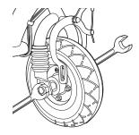
**2** Using two 17mm wrenches, loosen the front axle bolts by turning the wrenches counter clockwise. Remove wheel and install replacement wheel.
