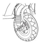
**1** Using a 10mm open wrench, loosen the brake cable bolt.
