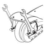
**1** Using two 13mm wrenches, loosen the rear axle bolts by turning the wrenches counter clockwise.
