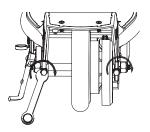
**2** Using a 10mm wrench, tighten the tension adjusters on the axle 1/8 to 1/4 turn to finetune the chain tension. Both adjusters must be tightened the exact same amount to maintain wheel alignment.
