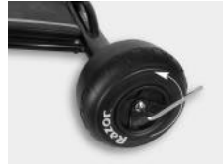
Figure 3e. Tightening the backwards threaded axle.
