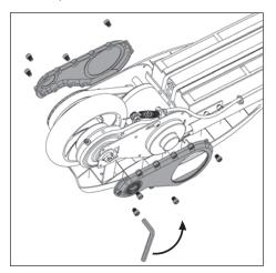
1. Using a 4mm hex wrench remove the 4 bolts from the rear axle cover on both sides of the scooter.
