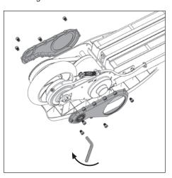
10. Reinstall side covers with a 4mm hex wrench. Do not over tighten bolts.
