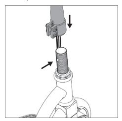
1. Depress the push button located on the rear of the fork and insert the handlebar steer tube onto the fork. The push button should align with the locator hole in the handlebar steer tube and lock the steer tube securely in place.
