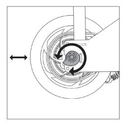
3. Rotate the adjustment washers against the frame tab to increase or decrease the belt tension. The recommended belt tension is based off of being able to twist the belt approximately 90 degrees.
