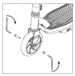
1. Using two 5mm hex wrenches loosen and remove the front axle by turning the wrenches counter clockwise.
