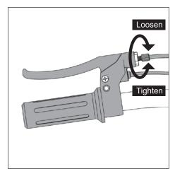
1. To adjust the brake cable thread clockwise (loosen) or counter clockwise (tighten) the adjuster barrel on the brake lever. Only turn the barrel in small increments until the desired adjustment is reached. If brake continues to need further adjustment proceed to the next step.
