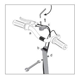
3. Align handlebars both vertically and horizontally (a) onto handlebar steer tube clamp (b) install handlebar clamp and hardware (c&d) and tighten evenly and securely with the 5mm hex wrench and 10mm wrench.
