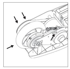
6. Install replacement wheel into the frame and slide belt back onto the pulley. Do not tighten axle nuts yet. Install brake arm hardware, do not tighten yet.
