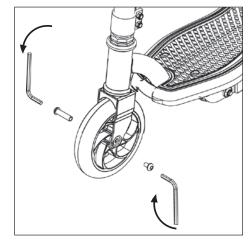
3. Reinstall hardware and tighten clockwise with a 5mm hex wrench.
