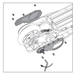
5. Reinstall side covers with a 4mm hex wrench. Do not over tighten bolts.
