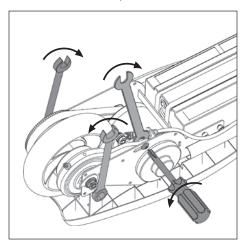
2. Loosen the brake arm bolt with a Phillips screwdriver & 10mm wrench. Using two 13mm wrenches loosen the rear wheel axle nuts.
