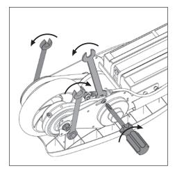
4. Ensure wheel is aligned in the frame and tighten the two axle nuts with a 13mm wrench. Retighten the brake arm bolt with a Phillips screwdriver.
