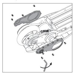
1. Using a 4mm hex wrench remove the 4 protective cover bolts on both sides of the scooter.
