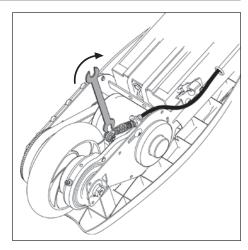
9. Retighten brake cable pinch nut with 10mm wrench. Refer to the instructions on page 7 for proper adjustment.
