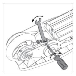
8. Retighten the brake arm bolt with a Phillips screwdriver & 10mm wrench.
