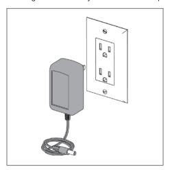
2. Plug the charger into a wall power outlet. The light on the charger housing should illuminate. Red LED light indicates battery is charging and a green LED light indicates battery is fully charged.
