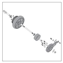
4. Note the location of all rear wheel hardware and ensure to properly reinstall all items.
