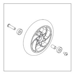
2. Reinstall new replacement wheel ensuring to note the order and location of all components.
