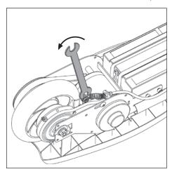
2. Loosen brake cable pinch nut with 10mm wrench.
