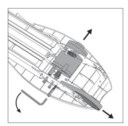
5. If replacing the belt remove the motor bolts with a 5mm hex wrench. Slide motor out of the frame slightly so that there is enough room to remove/replace the belt onto the motor gear. Replace spacers and retighten bolts.
