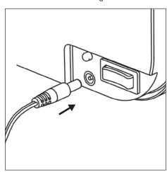
1. Make sure power switch is in the OFF position before plugging in the charger. Insert charger into charging port on the right side of the battery box.
