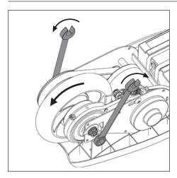
7. Ensure adjustment washers are seated correctly against the frame. After tightening axle nuts with a 13mm wrench check wheel alignment and the tracking of the belt by rotating the wheel counter clockwise with your hand. Adjustment washers may need to be readjusted to align belt. Refer to the instructions on page 10 for proper belt tensioning.
