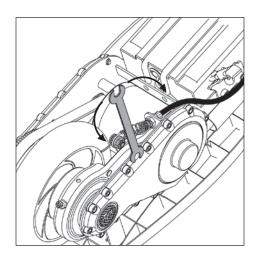
2. If the brake cable is still either too tight or too loose use a 10mm wrench to loosen the brake cable pinch bolt for further adjustment on the cable. Ensure that the 10mm nut is securely tightened after the adjustment is made.
