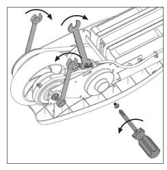
3. Remove the brake arm bolt with a Phillips screwdriver and 10mm wrench. Using two 13mm wrenches loosen the rear wheel axle nuts and adjustment washers and slide the belt off of the rear wheel pulley. Pull the wheel towards the rear of the frame.
