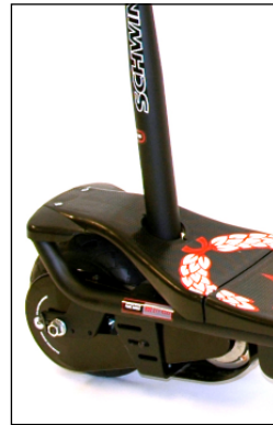
Drive train on the 300, 4.0 and 400 series scooters
