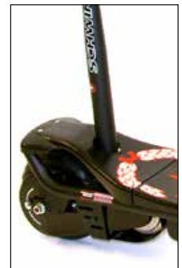
Drive train on the 300, 4.0 and 400 series scooters
