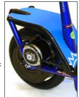
Drive train on the 500CD, 650CD, 750CD and 900CD series scooters
