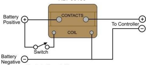
Contacts: Normally Open Maximum Continuous Contacts Load: 150 Amps
