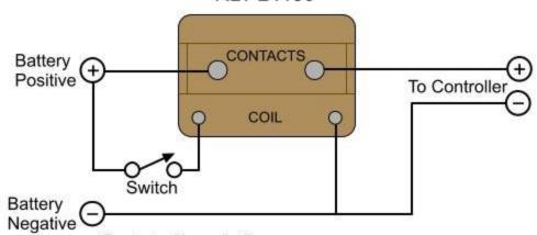
Contacts: Normally Open Maximum Continuous Contacts Load: 150 Amps
