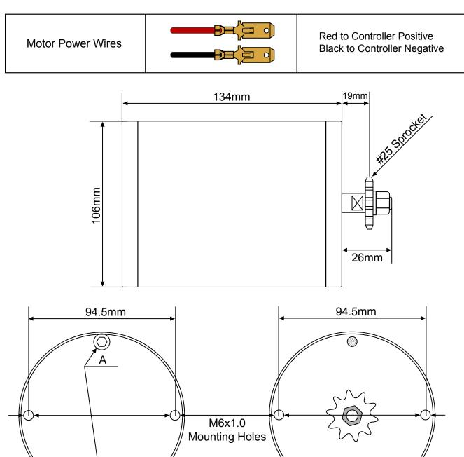
A = Recessed motor assembly bolts provide a flat backplate with no bolt heads protruding out of it.
